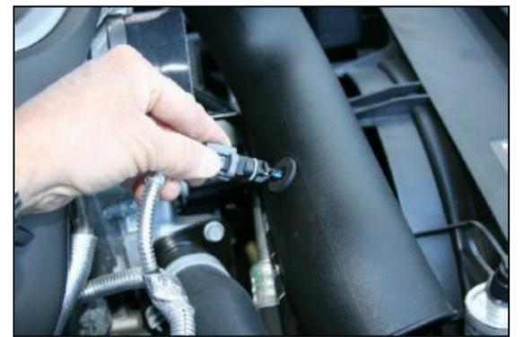
12. Carefully install the temperature sensor into the Airaid MIT as shown. Make sure it's pushed all the way in and the plug is connected to the wire harness.
