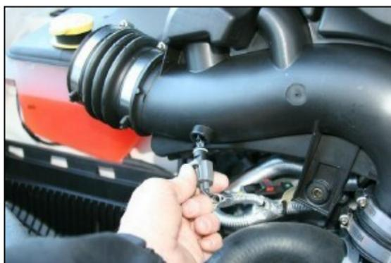
**7.** Carefully twist and remove the temperature sensor from the stock intake tube. Remove the stock intake tube from the vehicle.
