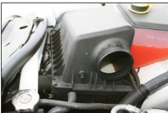
**8.** If you purchased an Airaid Jr. Kit, unhook the two clips and remove the factory air filter, and replace it with the Airaid Premium Filter supplied in the kit.
