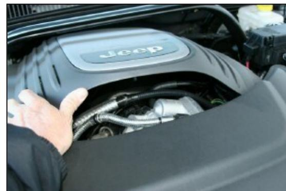
**3.** Carefully lift the engine cover for access to the throttle body. *(There are only grommets that hold down the cover, no bolts.)*
